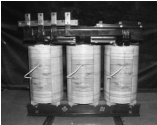
Fig.2 Transformer with layer wound coils
