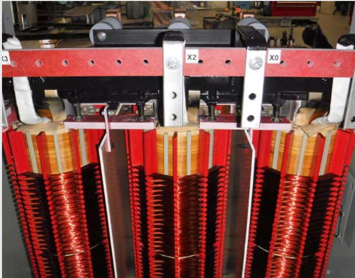
Medium Voltage Through 5 KV 600 Volt Class Secondary –3 Phase
