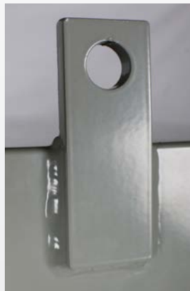
Two lifting lugs, fabricated from 3/8" x 1-1/2" stainless steel flat bar and welded to the top of the enclosure, are readily and permanently accessible.
